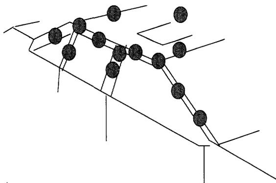
Figure 13. Target points defined in FMVSS 201.
