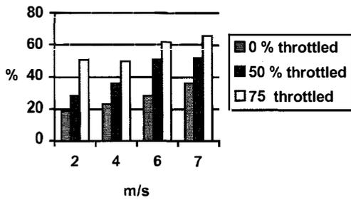
Figure 18. Energy absorption vs impact velocity, at different throttle rates.
