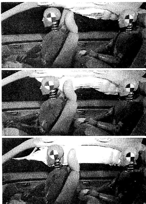
**Figure 10. IC deployment at 12, 17 and 24 ms, after ignition of the inflator.**
