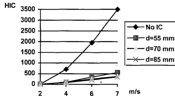
Figure 17. HIC vs velocity, at different cell thicknesses.
