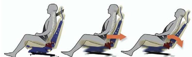
Figure 2. The recliner motion of WHIPS
