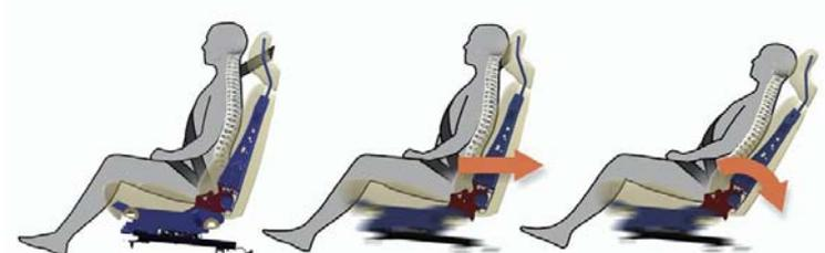
Figure 2. The recliner motion of WHIPS
