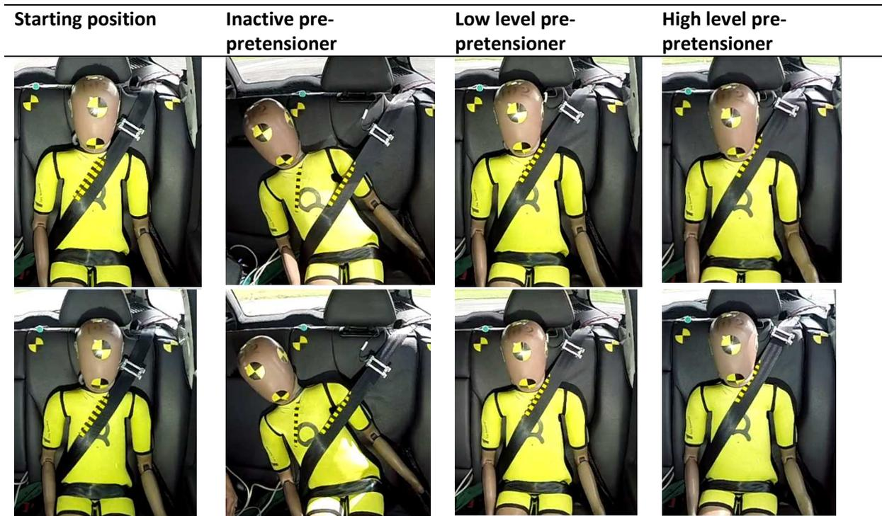
*Figure 1 The left column shows the starting positions of the Q6, the next three columns shows the maximum lateral inboard motion restrained without pre-pretensioner activation (second column), pre-pretensioner low level (third column) and pre-pretensioner high level (fourth column). The first row shows the first sequences of tests and the second row shows the repeated tests.*
