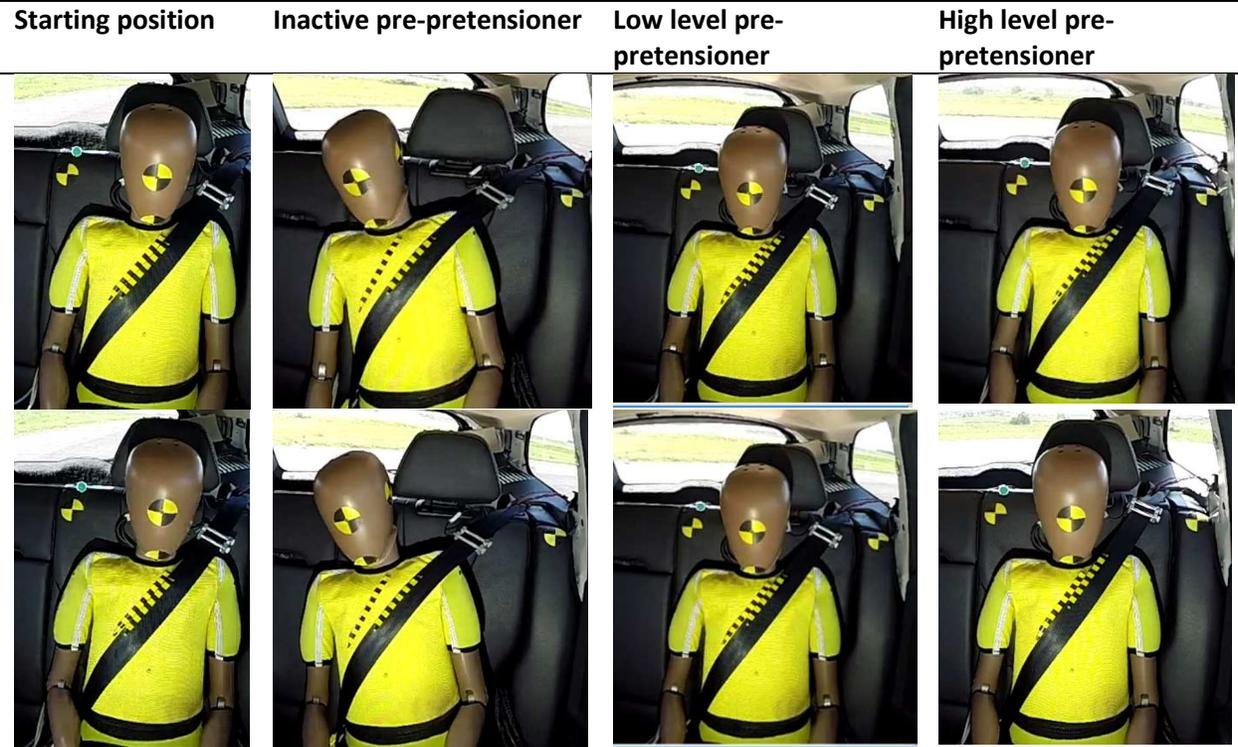
*Figure 2 The left column shows the starting positions of the Q10, the next three columns shows the maximum lateral inboard motion restrained without pre-pretensioner activation (second column), pre-pretensioner low level (third column) and pre-pretensioner high level (fourth column). The first row shows the first sequences of tests and the second row shows the repeated tests.*
