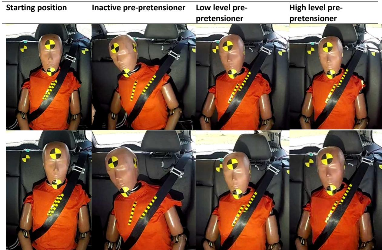
Figure 3 The left column shows the starting positions of the HIII5<sup>th</sup>, the next three columns shows the maximum lateral inboard motion restrained without pre-pretensioner activation (second column), pre-pretensioner low level (third column) and pre-pretensioner high level (fourth column). The first row shows the first sequences of tests and the second row shows the repeated tests.
