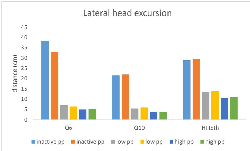
Figure 4 The lateral head excursion of the three ATDs, restrained without activation of pre-pretensioner (no pp), low level of pre-pretensioner force (low pp) and high level of pre-pretensioner force (high pp).
