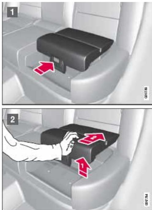
**Figure 7b. Folding function from low to high position.**
