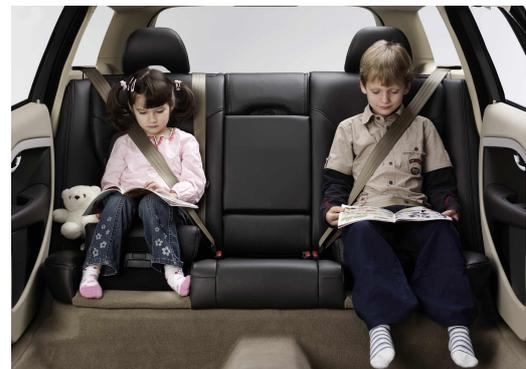
**Figure 6. Photo of two children using the 2-stage integrated boosters.**
