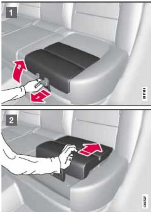
**Figure 7a. Folding function from folded down adult seat position to low position.**
