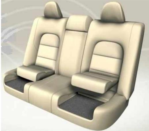
**Figure 4. The new 2-stage integrated booster cushion, low and high position, respectively**
