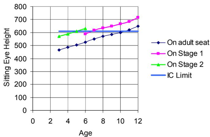
**Figure 4. Eye height for children when seated (50%-ile boys, ref Pheasant 1986). Horizontal line is the approximate level of the Inflatable Curtain (IC).**
