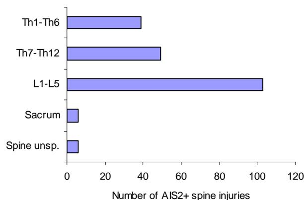
Figure 5. Number of AIS2+ injuries along the spine for the 189 occupants with 203 AIS2+ spinal injuries
