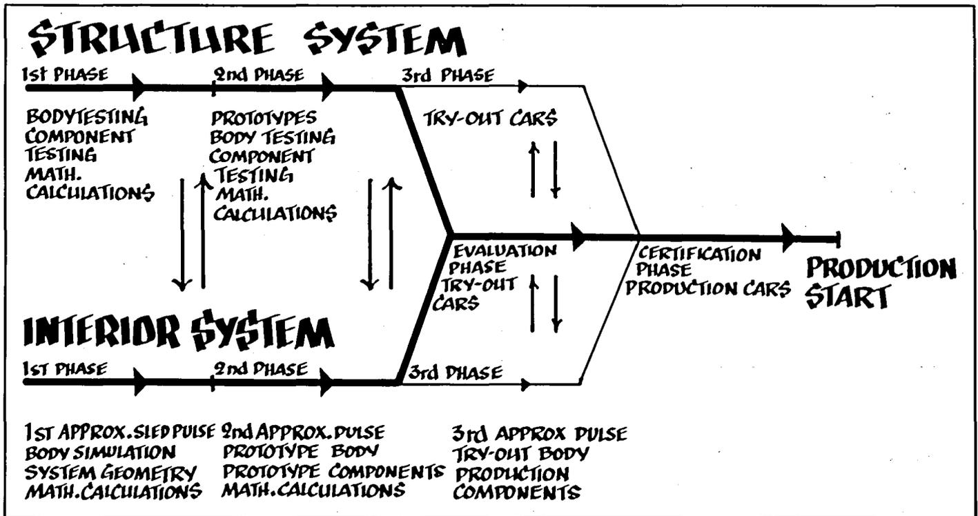
Figure 2. Development cycle for a new car.
