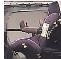
Figure 3b. Rearward facing seat, initial position (left) and maximum forward excursion (right).
