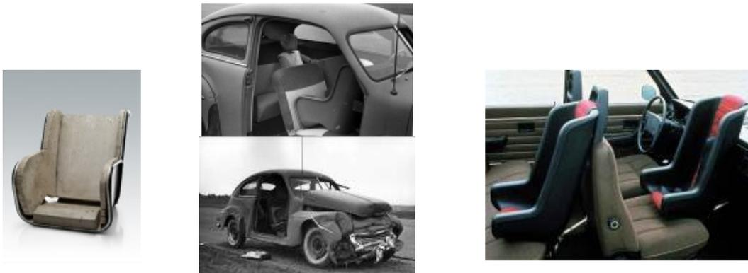
*Figure 1a. The first child seat prototype (child harness removed) by Prof. Bertil Aldman in 1964 (Aldman, 1964). Crash tested in a Volvo PV444.*
