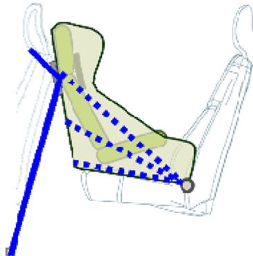
Figure 7b. Schematic restraint principles of concept CCS.
