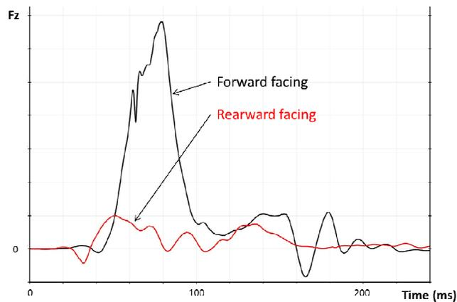
Figure 4. Upper neck tension force measured in a Q3 dummy, comparing forward facing and rearward facing seats during a severe frontal impact.
