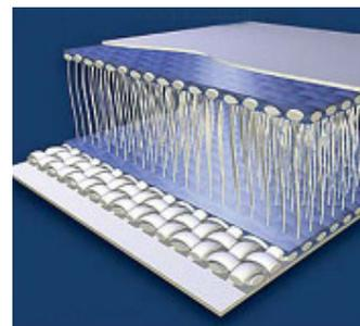
Figure 6b. Basic drop-stitch structural configuration.
