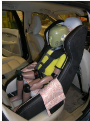
Figure 5b. CCS mounted in a passenger car with a Q3 dummy.
