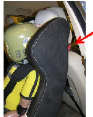
Figure 7c. Strap positioned around the front seat head restraint to secure support against the front seat.
