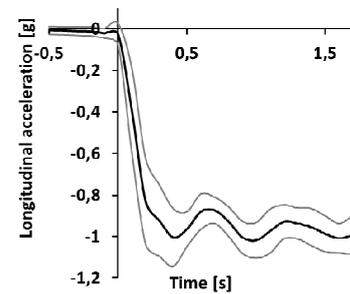
Figure 1c. Vehicle longitudinal acceleration during braking
