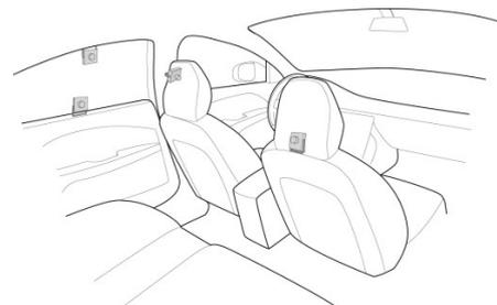
Figure 2c. Sketch of film camera placements
