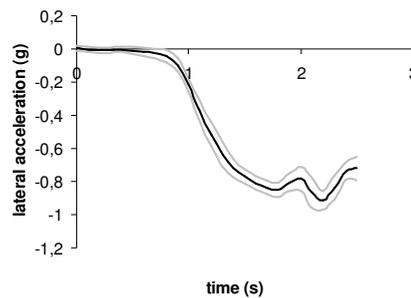
Figure 1b. Vehicle lateral acceleration during swerving manoeuvre
