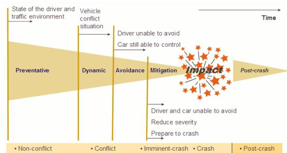
Figure 1. Phases leading up to an impact.
