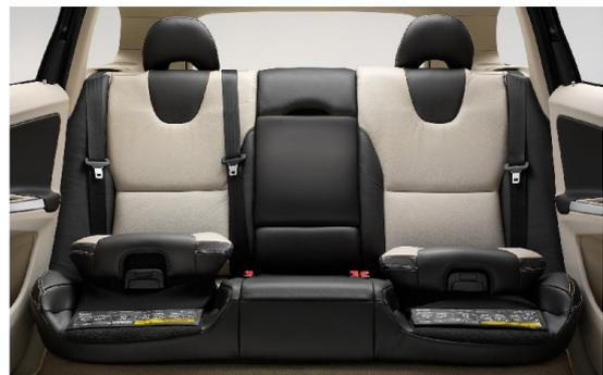
Figure 1c. Example of integrated boosters (2 stage)
