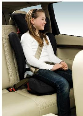
Figure 1b. Example of a high-back booster seat
